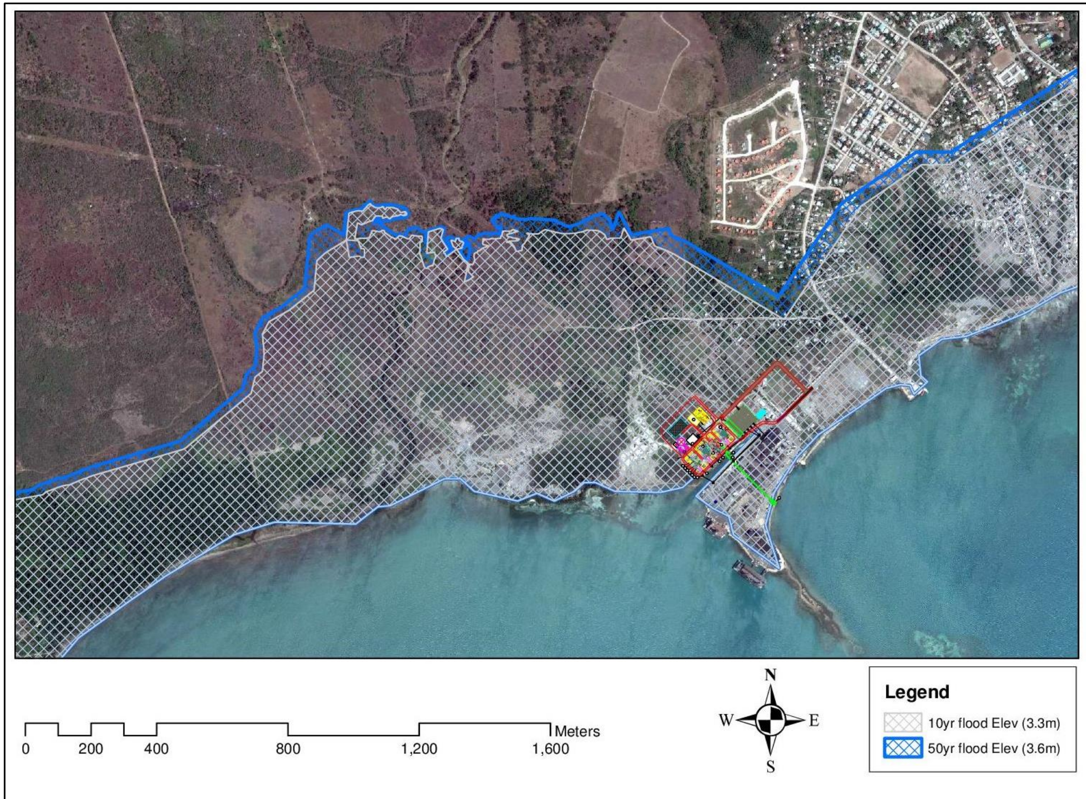
Figure 5-97 Storm Surge inundation Map showing the extents of the 10 year and 50 year storm surge incorrect map wrong site
